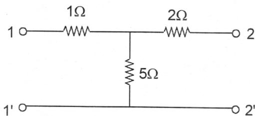
b) Calculate the characteristic impedance, the attenuation constant and phase constant of a symmetrical T network if -
