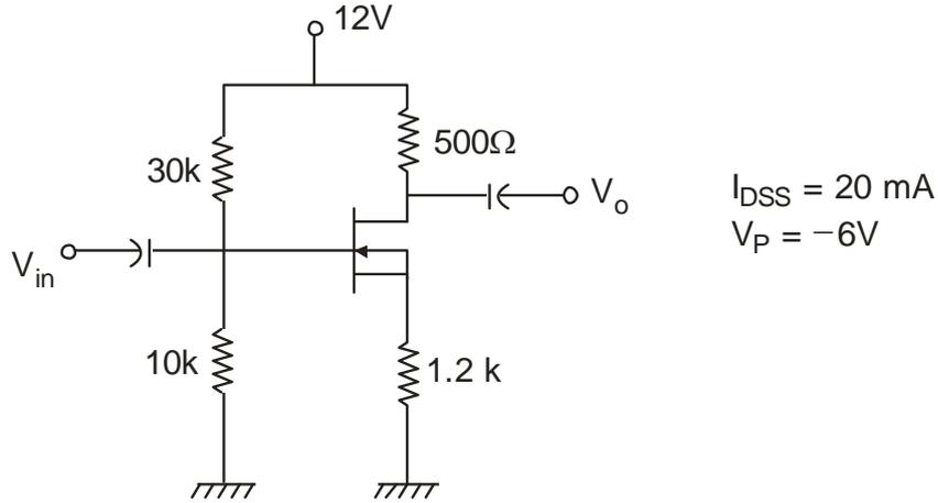
c) For the fig. shown below calculate  $g_m$ ,  $r_d$ ,  $Z_i$ ,  $Z_o$ ,  $A_v$  without  $r_d$  ( $R_F \geq r_d/R_D$ ,  $r_d \geq 10R_D$ ) 8
